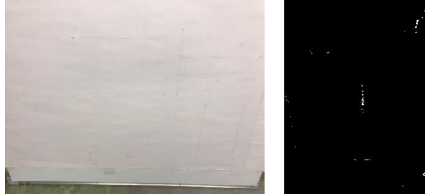
Fig. 15 Two obstacles with different reflectivity to be evaluated. Left: whiteboard (reflectivity 90%). Right: blackboard (reflectivity 10%)
